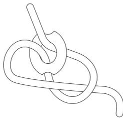
When the blind is raised, install the safety cleat and tie up the excess cord.
