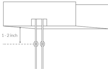
3. If cord-stops are not 1 to 2 inches below headrail, loosen (but do not untie) the knot surrounding the cord-stop.
